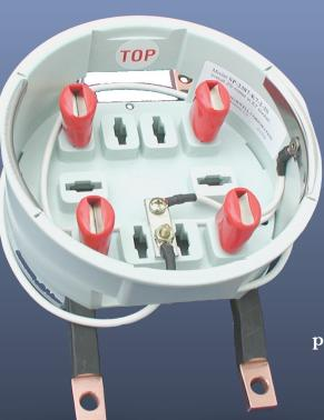
In the C&I sector, new "spec" buildings are often built with 400 amp or 600 amp polyphase bolt in meters. Later, when the building is leased it is sometimes determined that the meter and service panel are significantly oversized for the tenants expected load. The Marwell SP-2387-K7-2-2S adapter may be used to install a conventional residential single phase meter, class 200 or 320, at these sites.
