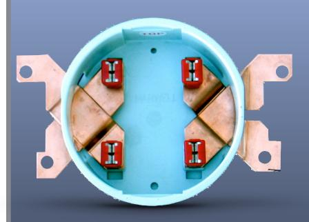
Marwell introduces another high quality product to add to our extensive line of K-Base conversion adapter products. The Marwell Corporation SP-2386-BF is the solution to the problem of bottom feed K-Base conversion. With the Marwell Corporation SP-2386- BF, you can safely use a Class 320 amp meter in a K-Base enclosure. Time tested Marwell adapter features, ensure safety and reliability in the critical application. Rated 400 Amp Max, 320 Amp Continuous. Assembled with UL recognized components.
